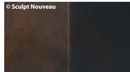
Birchwood Technologies M38 (left) and M24 (right) Patina applied hot to copper
